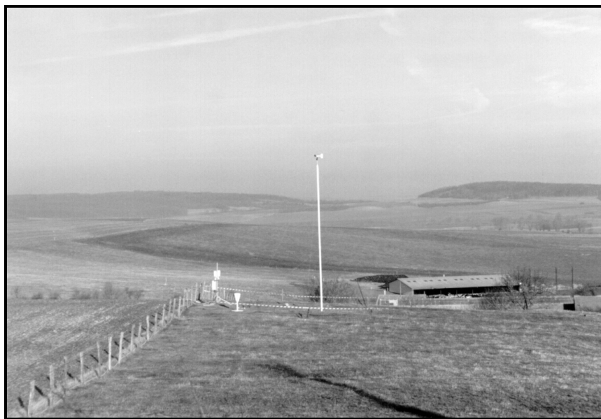
Photo 3 : General sight of the sensors from the building of the radar. From right-hand side to left side: the wind mast and its sensors, the rain gauge and the weather station on the ground.
